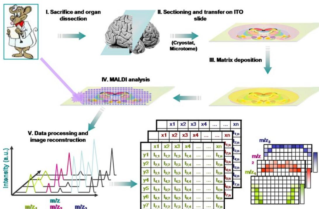
FIG. 1. **Schematic representation of the MALDI-MSI work flow.** After tissue sectioning and transfer onto a conductive and transparent sample plate, the MALDI matrix is deposited, and data are acquired by recording mass spectra according to a raster of points covering the surface to be analyzed. Mass spectra recorded with their coordinates on the tissue are processed, and molecular images of the localization of molecules can be reconstructed. *a.u.*, arbitrary units; *ITO*, indium tin oxide.
