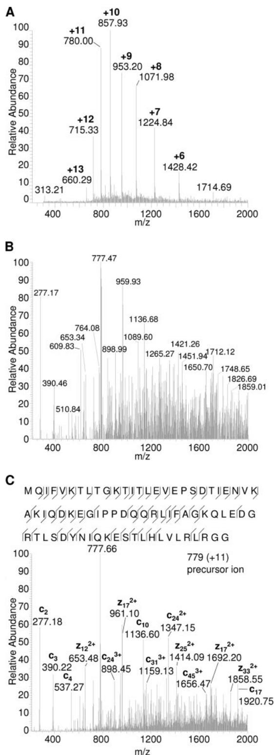
FIG. 4. A, the FF-TG AP-MALDI mass spectrum of a single scan acquisition from  $\sim 5$  pmol of ubiquitin in 2,5-DHB loaded onto the glass slide. B, the single scan ETD acquisition from the mass-selected 11+ charge state ( $m/z$  779) ions. C, the summed (40-s acquisition) proton transfer spectrum of the  $m/z$  779 ion with the sequence coverage shown.
